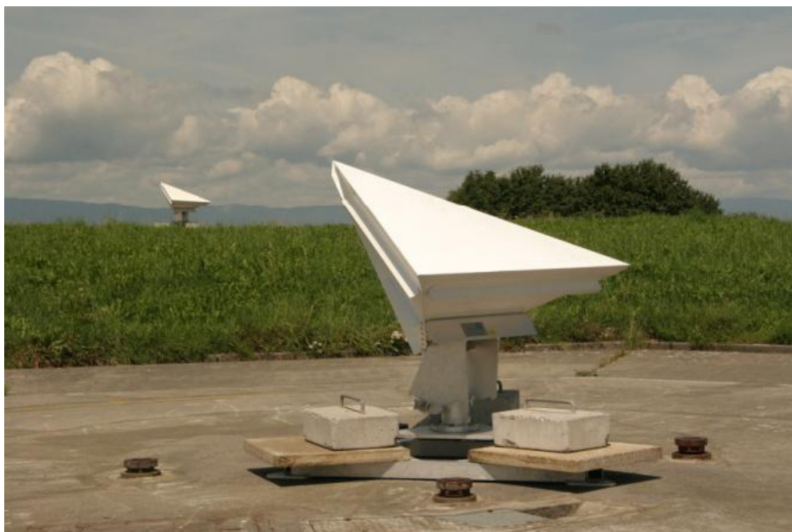
Figure 1. Trihedral corner reflectors in Torny-le-Grand facing TerraSAR-X's descending orbit.
