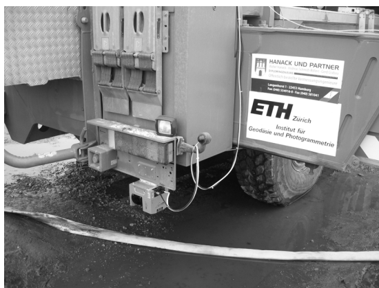
Figure 2. 2D-laser scanner mounted underneath the crane.
