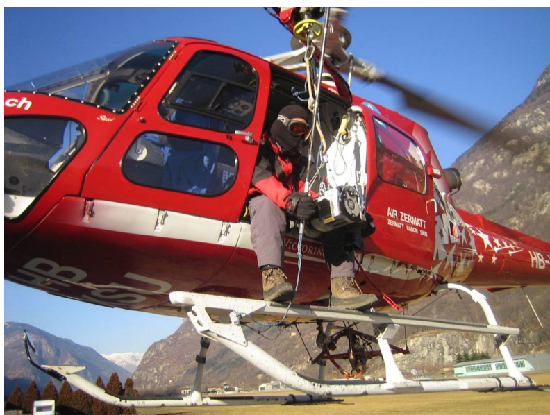
Figure 1. Handheld mapping system (Scan2map) installed in a helicopter.
