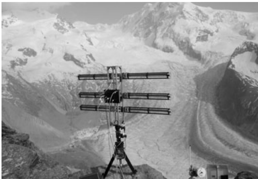
Figure 1. The portable radar interferometer deployed over the Gornerglacier showing the rotational scanner, antenna support structure, antennas, and microwave assembly.
