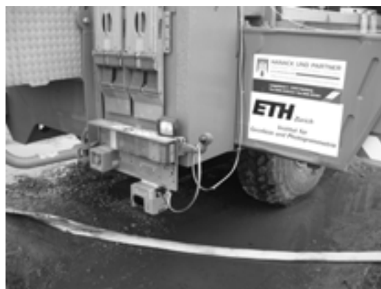
Figure 2. 2D-laser scanner mounted underneath the crane.
